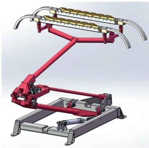
Fuente: Idun Truckled. (s.f.). Double arm railway pantograph design <https://www.iduntruckled.com/railway-pantograph/-double-arm-railway-pantograph-design.html>
